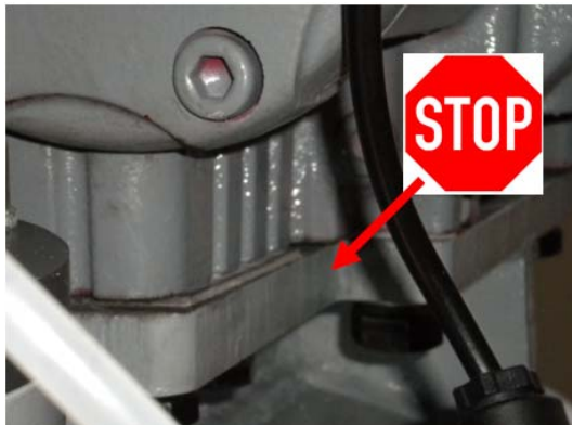
Bild: Wrong mounting of the air end
