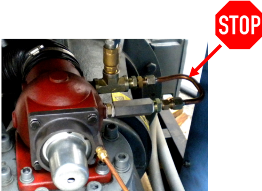
Fig: Wrong: Too small dimensioned piping for building up counter pressure for the rotors in oil-load.
