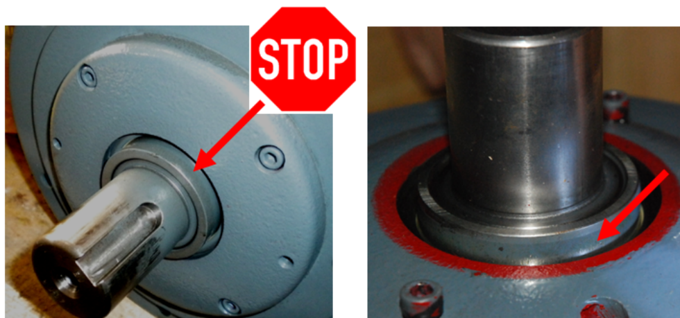
Fig: Protect the lip seal system by avoiding any foreign particles.
