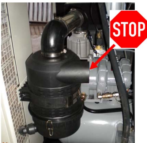
Fig: Suction pipe far away from hot temperature, and sources of dirt.
