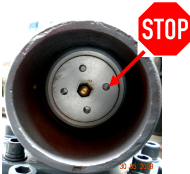
Fig: Avoid suction valve, which is closed 100% in off-load – apply bypass
