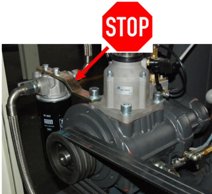
Fig: No mounting of additional parts to the airend, which can cause vibration.
