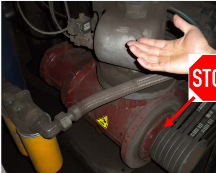
Fig: Protect the lip seal system by avoiding any foreign particles.
